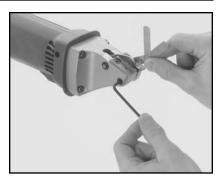
Figure 1. Setting gap with shims.
